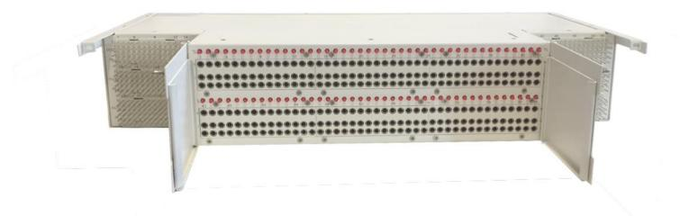
TXM's **DSX-LP-FX-84** is an 84 termination, front-split cross-connect DSX-1 panel for patching, terminating, and rearranging circuits using DS-1 (1.544 Mbps) or E1 (2.048 Mbps) signal rates.
